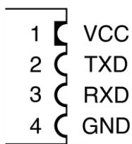
Figure 4. EPED003 ISO UART Micro Module Pin Diagram
